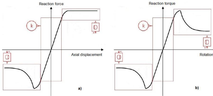
Figure 2: Constitutive sections of the reaction curves characterizing the joints of the Beam component. a) Reaction force / Axial displacement curve and b) Reaction torque / Rotation curve.
