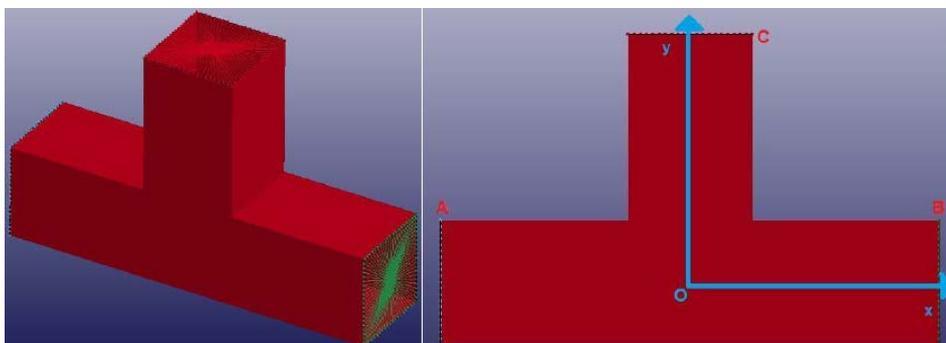
Figure 5: FE model of the three beam joint.
