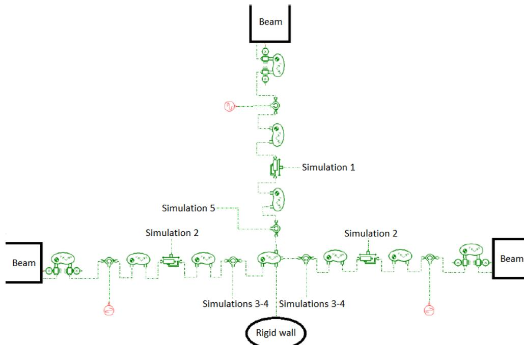
Figure 4: Schematic representation of a T-Joint component. The characteristic curves are assigned from different simulation cases at different points of the model.
