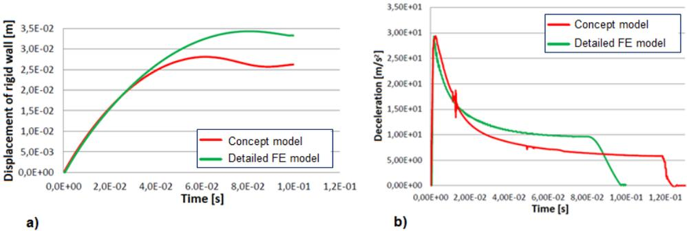
Figure 10: Comparison between the detailed FE model and the approximated model. a) Curve of displacement of the rigid wall with respect to time. b) Curve of deceleration of the rigid wall with respect to time.
