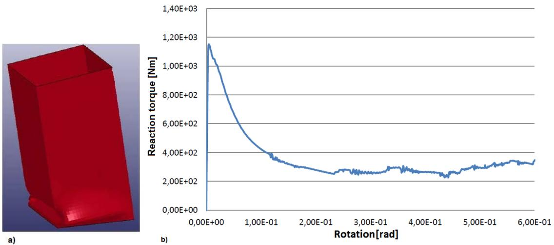
Figure 3: a) Deformation of the beam due to bending momentum and b) curve of reaction torque with respect to rotation.
