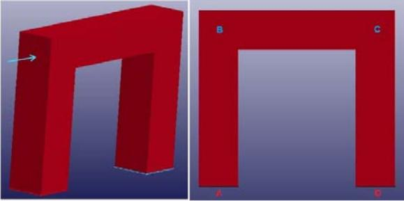
Figure 8: FE model of the C-shape structure.
