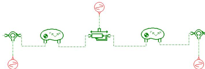
Figure 1: Schematic representation of a Beam component. A prismatic joint is in the middle coupling the two masses. At the other extremity of each mass a pivot joint is connected. The blocks in red contain the reaction curves of the joints.
