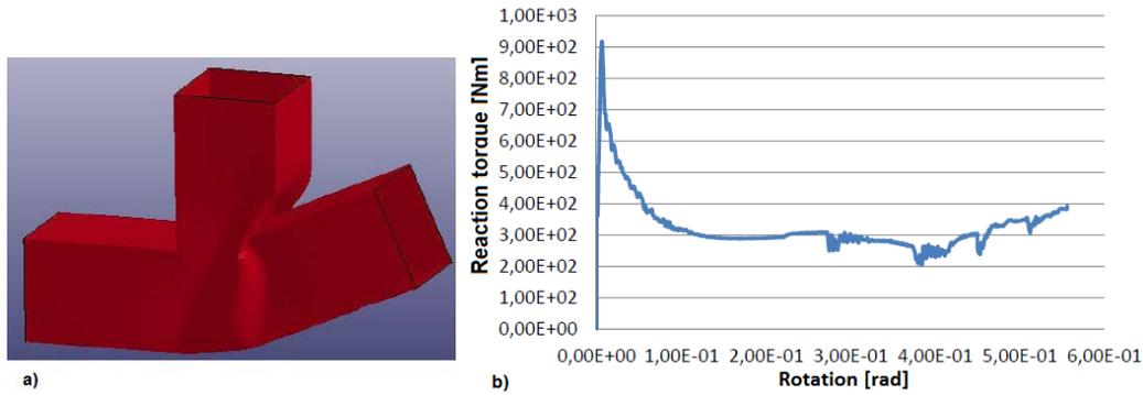
Figure 6: Simulation case of a rigid wall of 750 Kg impacting at one end of the T-joint with initial speed of 1 m/s. The other two ends are clamped to observe the generation of a plastic fold close to the point of intersection of the three beams. a) Final deformation. b) Corresponding reaction torque/rotation curve.
