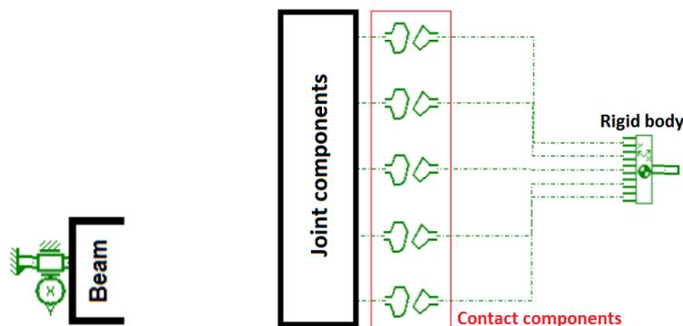
Figure 7: Schematic representation of Boundary Condition components. Left: Clamp component. Right: Rigid Wall component.
