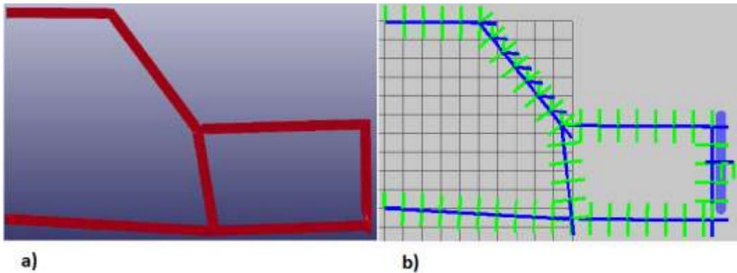
Figure 14: Visual comparison of the deformation on the a) detailed FE simulation and the b) concept model.
