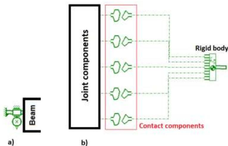
Figure 6: Schematic representation of Boundary Condition components.
