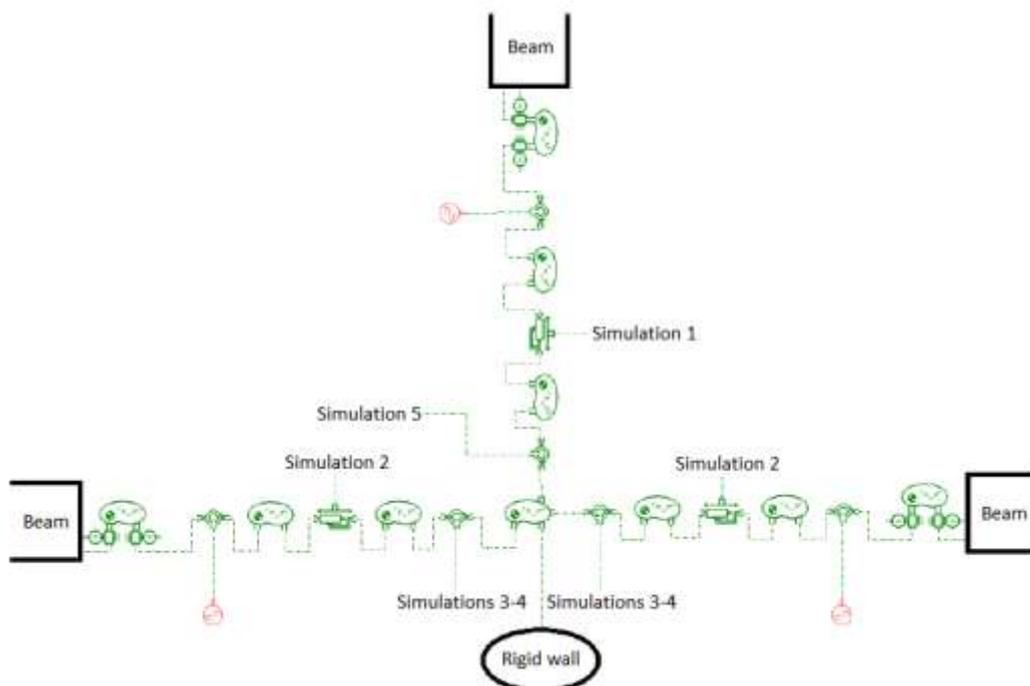
Figure 3: Schematic representation of a T-Joint component. The characteristic curves are assigned from different simulation cases at different points of the model.
