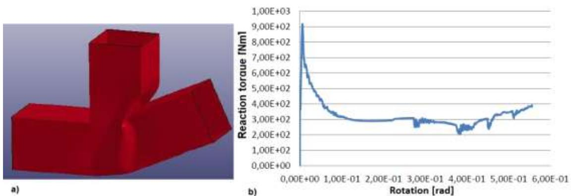
Figure 5: Simulation case of a rigid wall of 750 Kg impacting at one end of the T-joint with initial speed of 1 m/s. The other two ends are clamped to observe the generation of a plastic fold close to the point of intersection of the three beams. a) Final deformation. b) Corresponding reaction torque/rotation curve.
