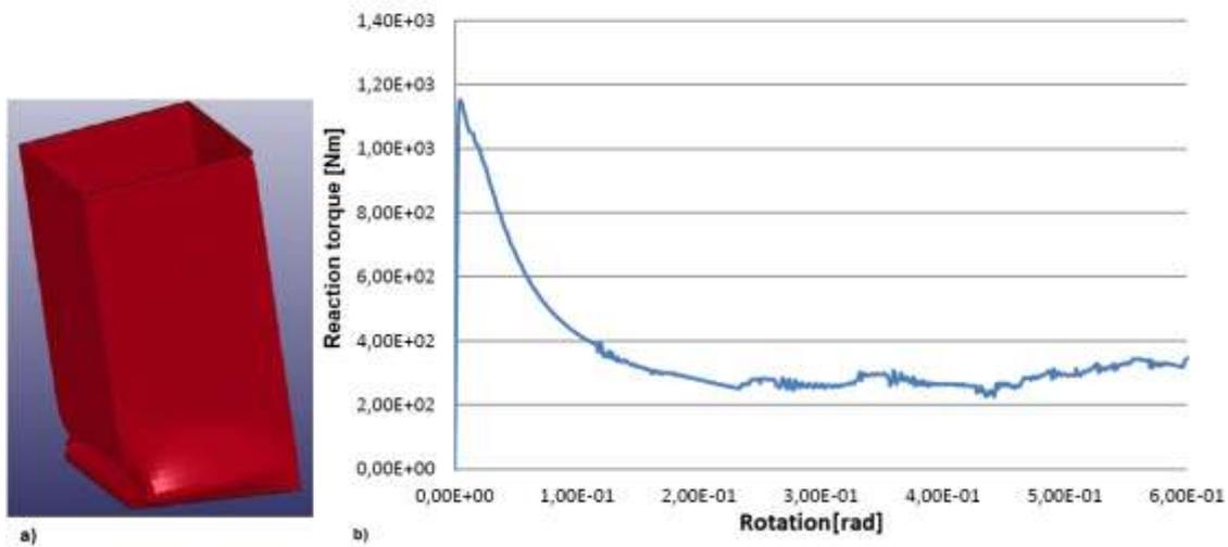
Figure 2: a) Deformation of the beam due to bending torque and b) curve of reaction torque with respect to rotation.
