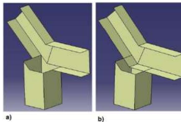
Figure 11: Modification of the critical part 1. a) Original part and b) stiffened part.
