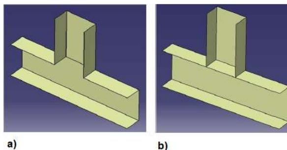
Figure 12: Modification of the critical part 2. a) Original part and b) stiffened part.
