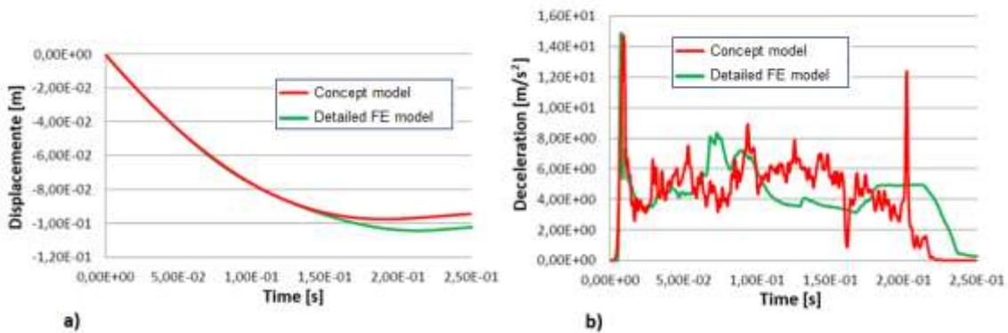
Figure 8: Comparison between the detailed FE model and the concept model. a) Curve of displacement of the rigid wall with respect to time. b) Curve of deceleration of the rigid wall with respect to time.
