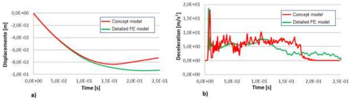
Figure 13: Comparison between the detailed FE model and the concept model. a) Curve of displacement of the rigid wall with respect to time. b) Curve of deceleration of the rigid wall with respect to time.
