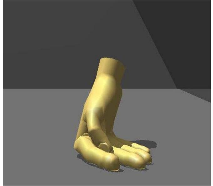
Fig. 3. Self-collision between thumb and other fingers.
