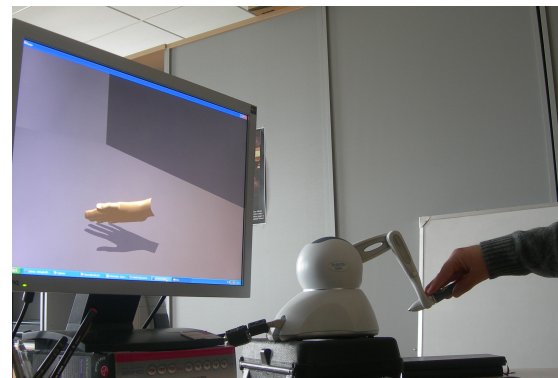
Figure 1: Haptic manipulation of a virtual hand.
